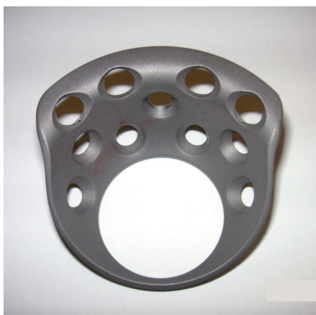
Figure 1. The ARR (view inside the ring). In the present study, ARRs made of steel and ARRs made of titanium were used. The shape remained the same.
