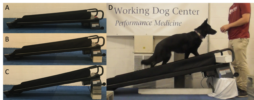
Figure 1. (A) 2% incline treadmill without elevation. (B) 10% incline treadmill elevated to 10 cm. (C) 20% incline treadmill elevated to 25 cm. (D) Dog performing an acclimation session on the full 20% incline treadmill setup.
