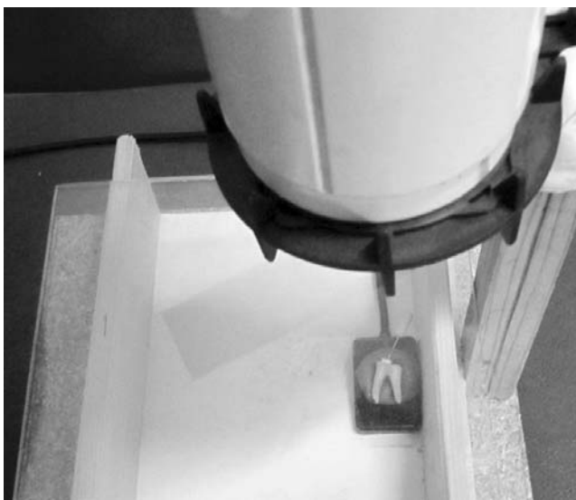
Fig. 1. Right angle direction of central ray toward the image receptor and tooth by film holder and prefabricated apparatus.
