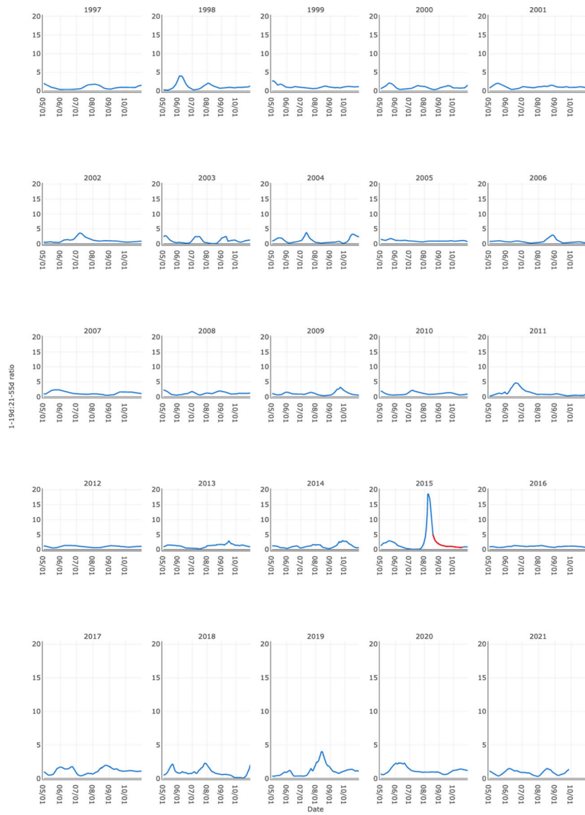
Figure 4. Yearly plots of the ratio of the 1 to 19 day and 21 to 55 day average lagged exceedances at Pike Island.
