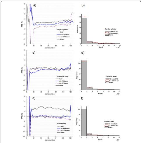
**Fig. 4** RPD of NAC, TX-based AC, and CT-based AC PET images for the acrylic cylinder, posterior array, and patient table are shown in **a**, **c** and **e**, respectively, compared to blank. Distribution of photon counts are displayed in histograms in **b**, **d**, and **f** comparing TX-based AC to CT-based AC and blank
