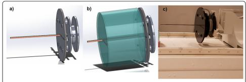
**Fig. 1** The apparatus (TX-fixture) and setting used in PET acquisitions, **a** schematic of the TX-fixture showing the radioactive Ge-68 rod positioned in the centre, during blank scan, **b** both the acrylic cylinder phantom and the rod attached to the TX-fixture, and **c** the QC-daily phantom holder securing the TX-fixture to achieve a reproducible position on the patient table
