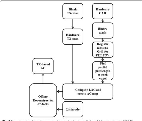
**Fig. 2** Flow chart describing the process of generating hardware TX-based AC map using the PET/MRI scanner and a static radioactive source
