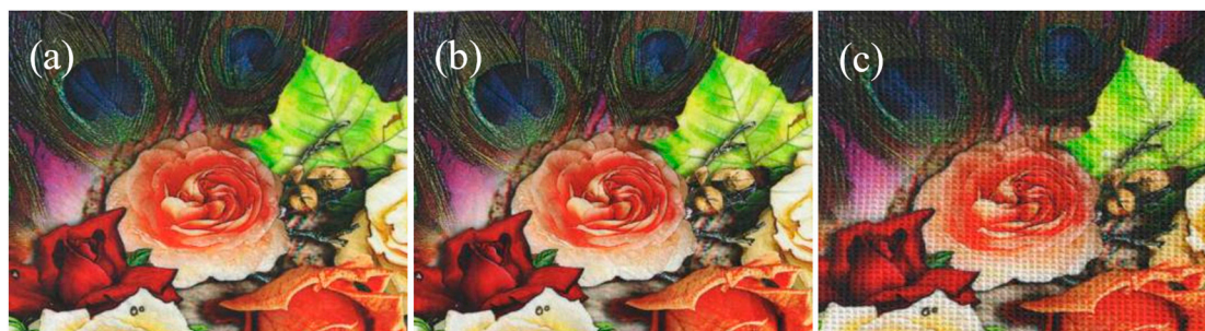
Figure 8. Scanned images of ink-jet printed plain fabrics (a), twill fabrics (b), and honeycomb fabrics (c). All fabrics were padded through modification fluid (1 g/L of nanospheres and 10 g/L of sodium bicarbonate) steamed at 102 \pm 1 °C for 6 min.
