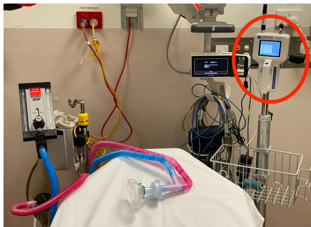
Fig. 1 Particle counter (circled in red) positioned at the head of the bed to simulate staff member face level.
