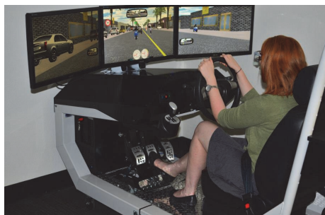
FIGURE 1: The Curtin University STISIM driving simulator.
