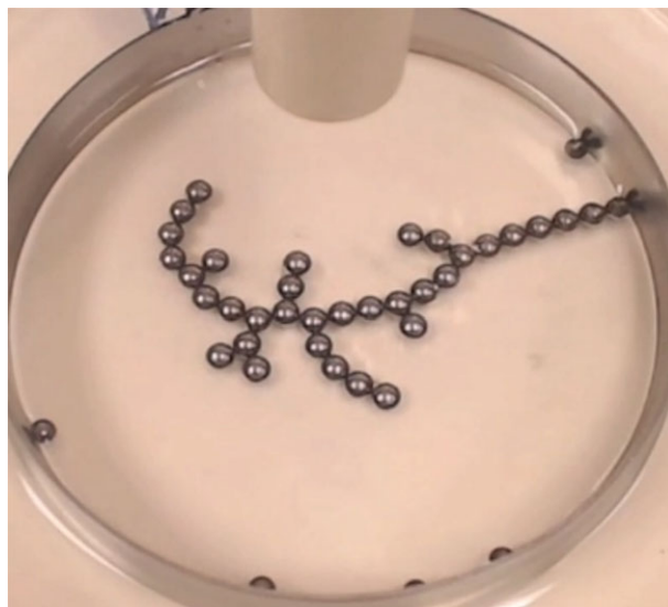
Figure 1. A ramified charge-transportation network (RCTN). When conductive chromium spheres are partially submerged in oil and subjected to a high voltage potential, they self-organize into dendritic structures such as that shown here. In this experiment [1], the spheres are 4 mm in diameter. Image used with permission of its creators.
