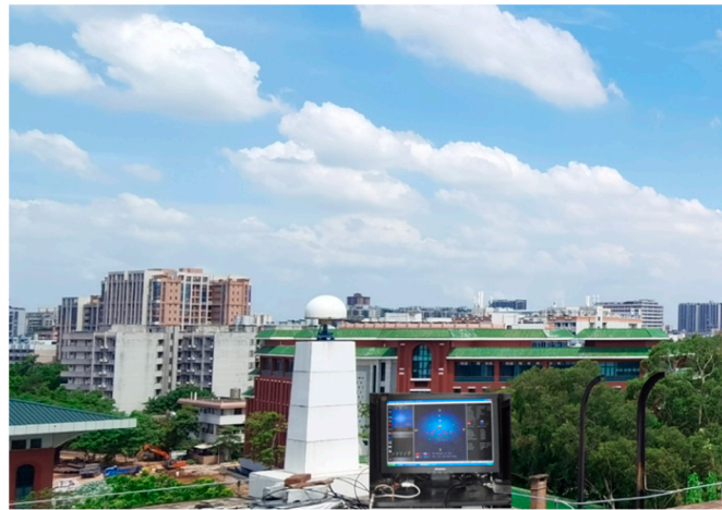
Figure 21. Base station for DGNSS experiment on SYSU campus.
