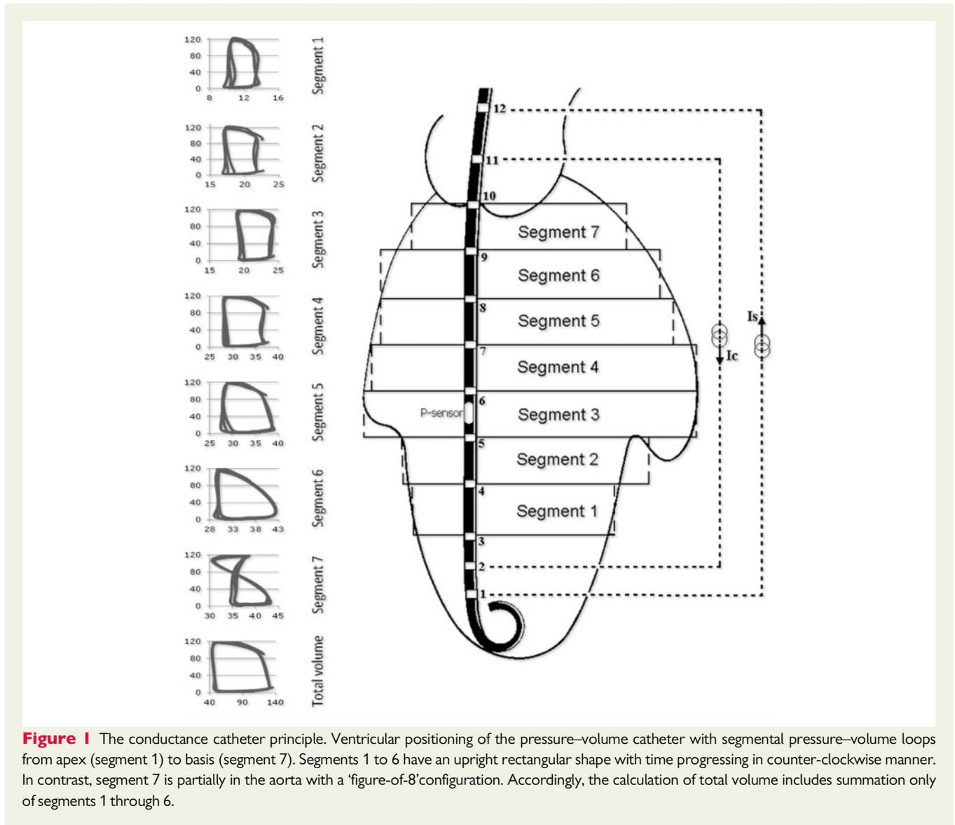
**Figure 1** The conductance catheter principle. Ventricular positioning of the pressure–volume catheter with segmental pressure–volume loops from apex (segment 1) to basis (segment 7). Segments 1 to 6 have an upright rectangular shape with time progressing in counter-clockwise manner. In contrast, segment 7 is partially in the aorta with a ‘figure-of-8’ configuration. Accordingly, the calculation of total volume includes summation only of segments 1 through 6.
