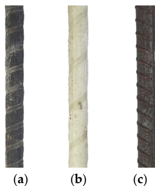
Figure 1. Reinforcement bars: (a) BFRP bar; (b) GFRP bar; (c) Steel bar.
