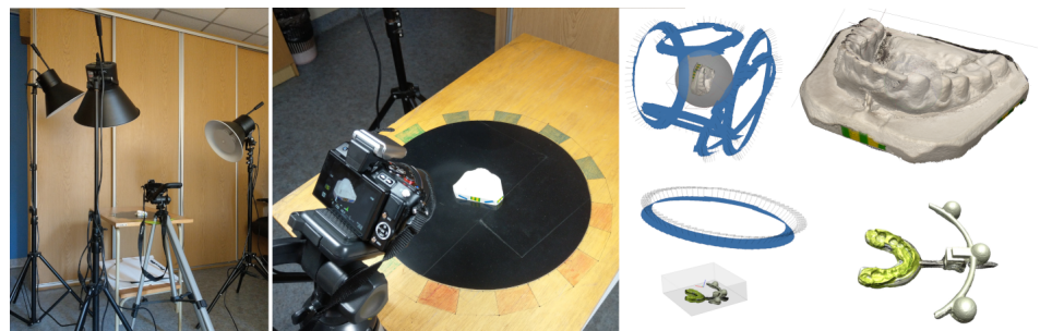
Figure 4. Left and centre: photographing a dental model. Right: camera positions while shooting and the reconstructed digital models.
