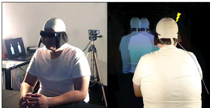
Fig. 1 Stereoscopic 3D full-body illusion combined with HD-tDCS. Front (L) and back (R) view of full-body illusion paradigm based on LIVE-streaming stereoscopic 3D images with Bino 3D Player (Lambers, 2012), here combined with high-definition transcranial direct current stimulation (HD-tDCS). The DC Stimulator Plus (neuroConn) can be seen to the side of the participant fastened on top of a table.
