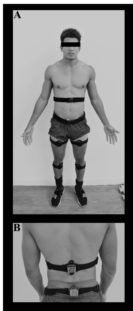
Figure 4. Inertial sensor placement: (A) front view; (B) back view.
