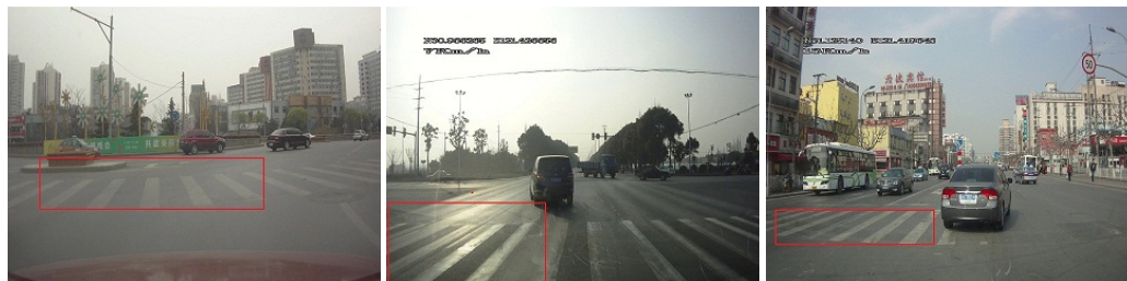
(a) Examples of detection results for one pedestrian crossing.
