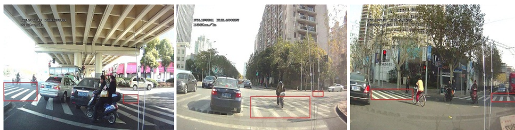
(b) Examples of detection results for two pedestrian crossings.
