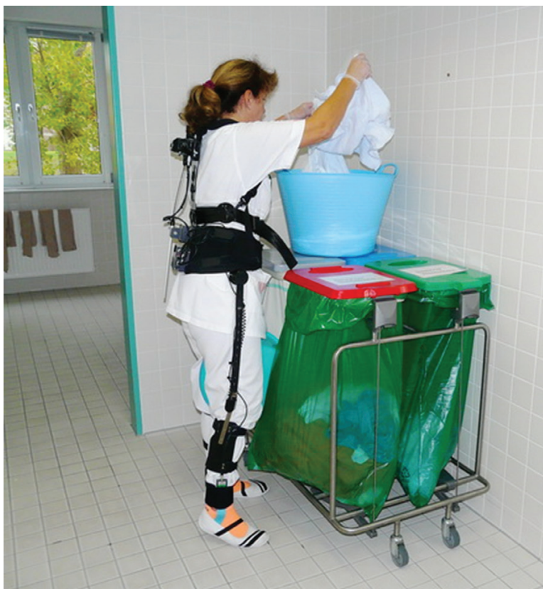
Figure 1. A nurse is wearing the CUELA measurement system while working. Sensors on the thoracic and lumbar spine deliver three-dimensional data on trunk movements.
