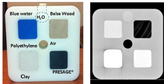
FIG. 3. HU-RLSP phantom and CT image of the phantom.
