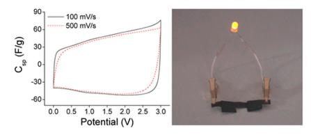
**Figure 7.** Characteristics of CNT/BNC/ion gel-based all-state flexible supercapacitors. The left figure shows cyclic voltammetry (CV) curves measured at scan rates of 100 and 500 mV/s. The right figure shows a photograph of a light-emitting diode (LED) turned on by the flexible supercapacitors. Reproduced with permission from [120]. Copyright American Chemical Society, 2013.
