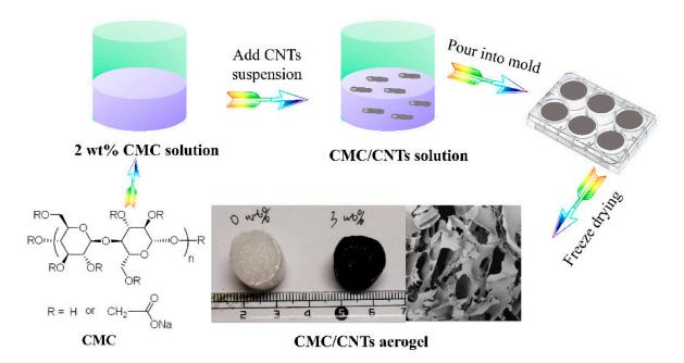
**Figure 4.** Preparation of CMC/CNTs aerogel. Reproduced with permission from [84]. Copyright MDPI, 2019.
