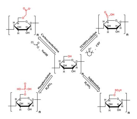
**Figure 2.** Different surface modification techniques through which ionic charges are imparted to the NC surface. Reproduced with permission from [20]. Copyright American Chemical Society, 2018.
