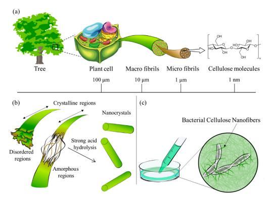
**Figure 1.** Cellulose contained in plants or trees has a hierarchical structure from the meter to the nanometer scale, as shown in (**a**). A schematic diagram of the reaction between cellulose and strong acid to obtain Nanocellulose is shown in (**b**). Bionanocellulose cultured from cellulose-synthesizing bacteria is shown in (**c**). Figure 1 was drawn by co-author R. Hamano.
