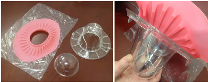
FIG. 4. (Left) a photo of the pink flange, inner cup, and outer cup. (Right) the all three pieces assembled.
