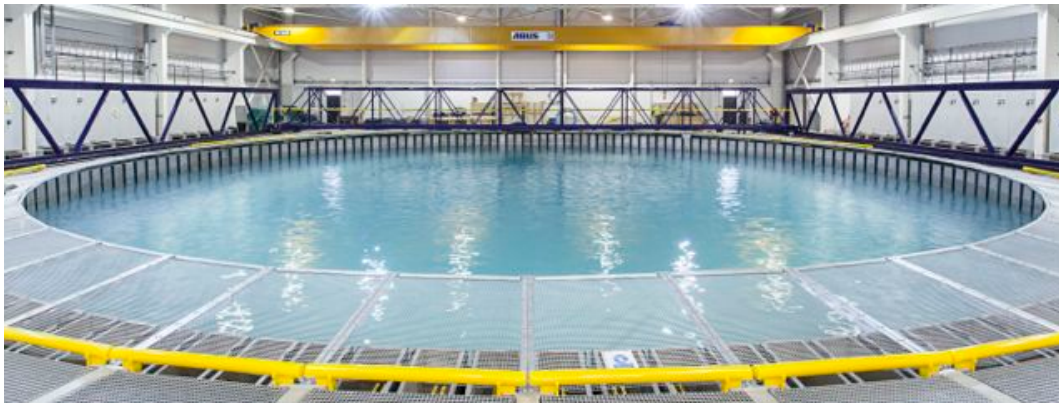
Figure 1. The Flowave Ocean Energy research facility - a circular wave and current test tank of 25 m diameter and a working depth of 2 m.
