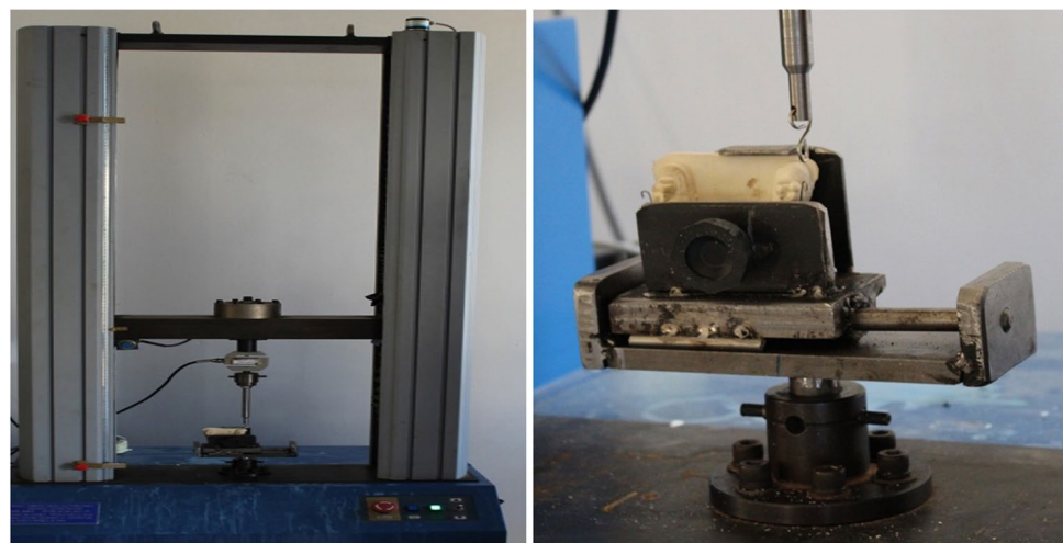
Fig. 2 The universal mechanical testing machine used in the frictional analysis
