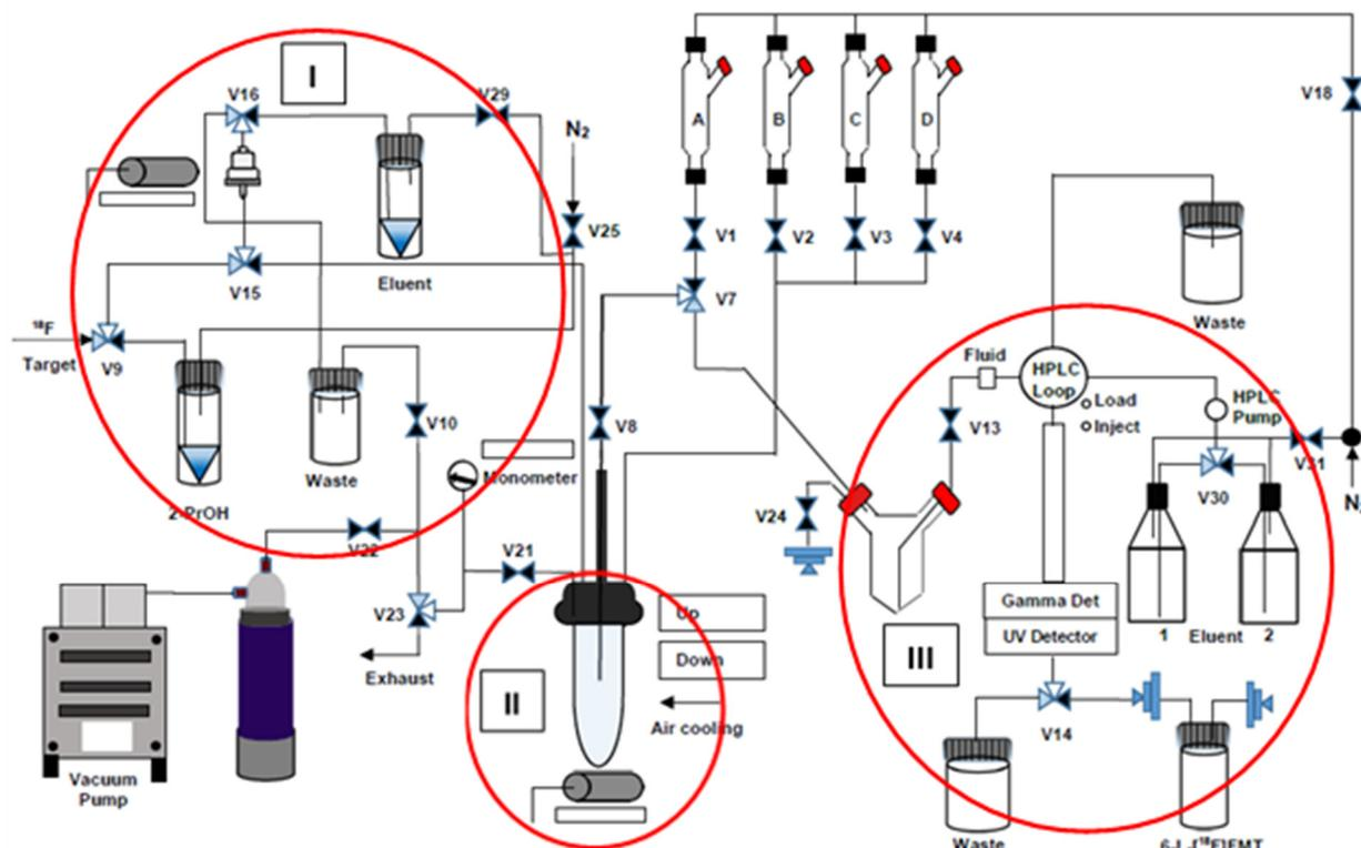
**Figure 5.** Schematic diagram of the GE TRACERlab FX-C Pro module modified for the preparation of 6-L-[<sup>18</sup>F]FMT. A: empty vessel; B: 0.5 N HCl in 50% MeOH (1 mL); C: MeOH (0.5 mL); D: 0.1% AcOH (1.5 mL); RV: **4** (7.7 mg, 10 μmol) and Cu(py)<sub>4</sub>(OTf)<sub>2</sub> (11 mg, 16 μmol) in MeCN (0.3 mL); eluent vial: Bu<sub>4</sub>NOTf (5 mg, 12.5 μmol) in *i*PrOH (0.8 mL). RV—reaction vessel (2 mL).
