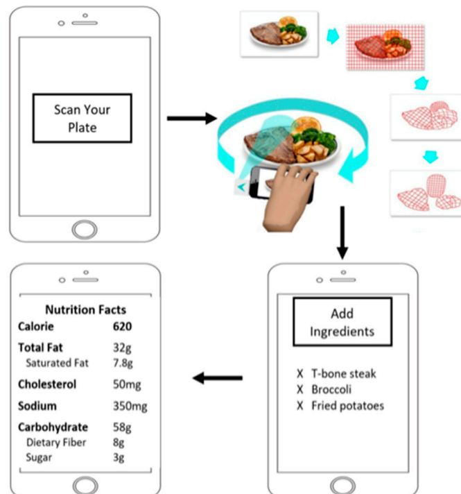
Figure 2. The overall DDRS system and the smartphone application. Starting from the top left, once the user starts the scanning process and the ingredients are added, the nutritional facts are generated based on the amount of food scanned.
