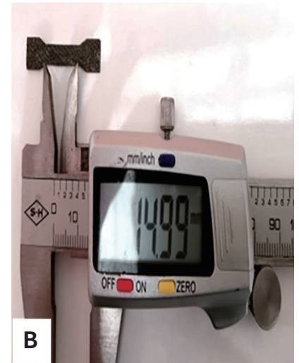
Fig. 1. Dog-bone shaped tensile test sample. (A) Diagram of the shape and dimensions of the dog-bone sample. (B) DMLS printed tensile test sample.
