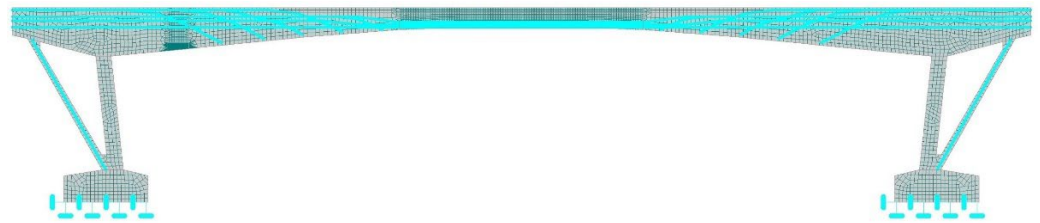
Figure 16. FE model in ATENA 2D Software.
