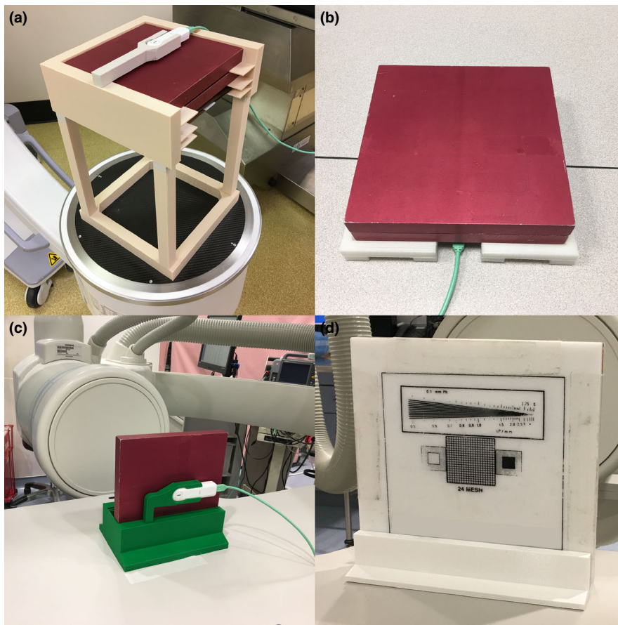
FIG. 4. Positioning aids for (a) portable c-arm fluoroscopes, (b) R/F rooms with under-table x-ray tube, (c) interventional c-arms in the lateral position, and (d) an image quality phantom holder for use in fluoroscopy or radiography.
