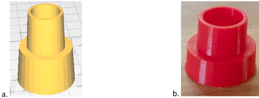
Fig. 3. a) Rendering of the hose adaptor, b) 3-D printed hose adaptor.
