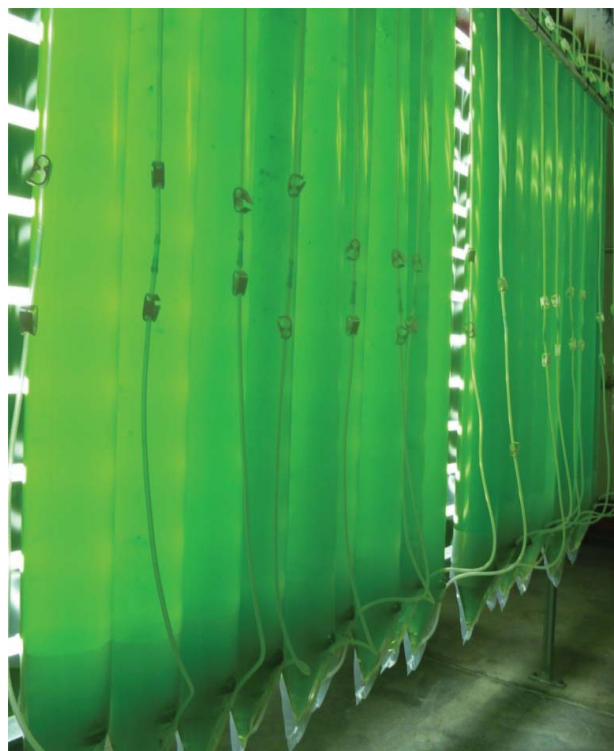
Figure 1. A low-cost, single-use photobioreactor system for commercial production of algal biomass. This ‘hanging bag’ system was developed by the Cawthron Institute, New Zealand for production of microalgae as aquaculture feed and for cultivation of Haematococcus pluvialis – a natural source of the high-value nutraceutical astaxanthin. We have successfully adapted the system for endolysin and vaccine production in C. reinhardtii (L. Stoffels, B. Parker and S. Purton, submitted). The 40 litre bags are optimally illuminated and sterile 5% CO 2 /95% air supplied at the base of each bag for phototrophic growth and for mixing. Both batch and continuous operation is possible. ©Supreme Health, New Zealand. Reproduced by permission of Supreme Health, New Zealand. Permission to reuse must be obtained from the rightsholder.
