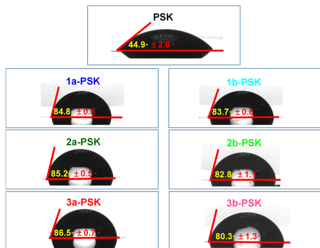
Figure 11. Water contact angles of pristine, 1a–1b , 2a–2b , and 3a–3b -treated perovskite films.
