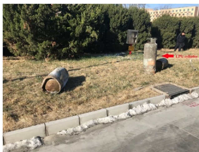
Figure 6. LPG cylinders after the explosion (damaged).
