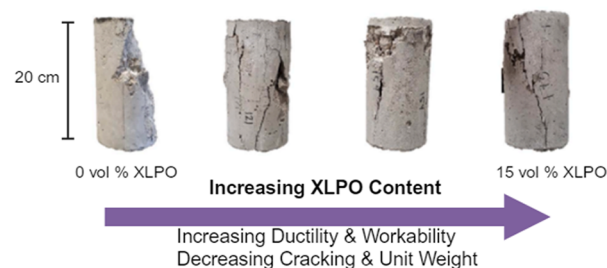
Figure 6. Photographs of representative failed concrete samples from a uniaxial compression test with XLPO content varied from 0 to 15 vol %. Concrete cylinders were prepared at a water-to-cement fraction by mass of 0.50, and compression tests were conducted according to ASTM C39. Higher XLPO contents led to more ductile and workable concrete that was less susceptible to cracking. Adapted with permission from ref 72. Copyright 2024 Elsevier.
