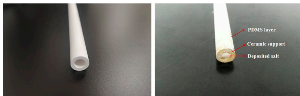
Figure 5. Virgin (left) and fouled (right) PDMS/ceramic tubular membranes.
