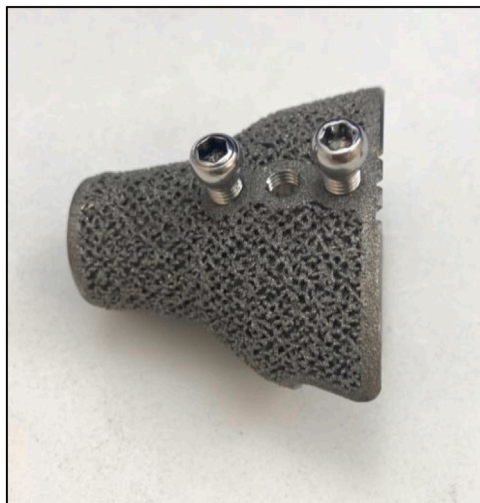
Figure 1. Porous custom-made cone for metaphyseal tibia bone loss with screws for tibial tubercle osteotomy fixation.
