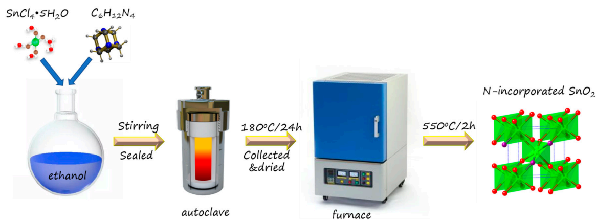
Figure 1. Scheme of the synthesis process of N-incorporated SnO 2 nanostructure.
