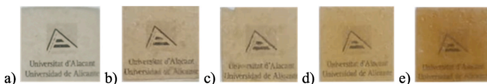
Fig. 1. Aspect of the sheets obtained; a) 60TPS, b) 60TPS-0.5 GA, c) 60TPS-1GA, d) 60TPS-2GA and e) 60TPS-5GA.
