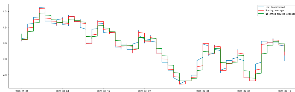
Figure 1. The log-transformed, moving average and weighted moving average of NO 2 concentration datasets.
