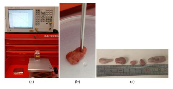
**Figure 1.** (a) Dielectric measurement setup: the open-ended coaxial-probe is connected with a right angle SMA-connector to a vector network analyzer during the measurement of the validation load (0.1 Molar NaCl water solution). (b) Detail of a human axillary lymph node measurement. (c) Five sheep inguinal lymph nodes that have been measured.
