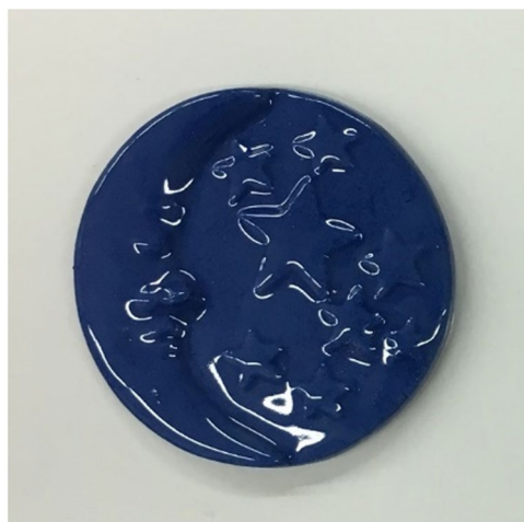
Figure 7. Coloured porcelain body obtained with 10% of zeolite based cobalt pigment.
