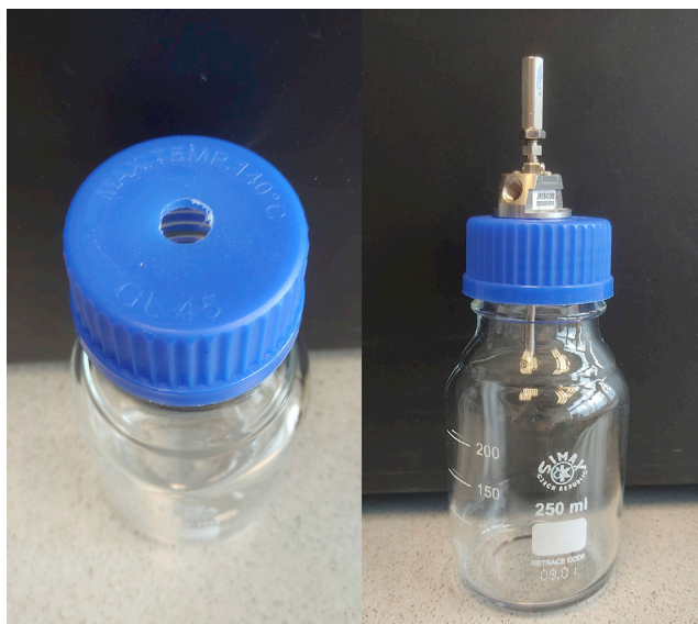
Figure 1. Waste container and holder for the spray needle during the passivation of the HPLC-MS system
