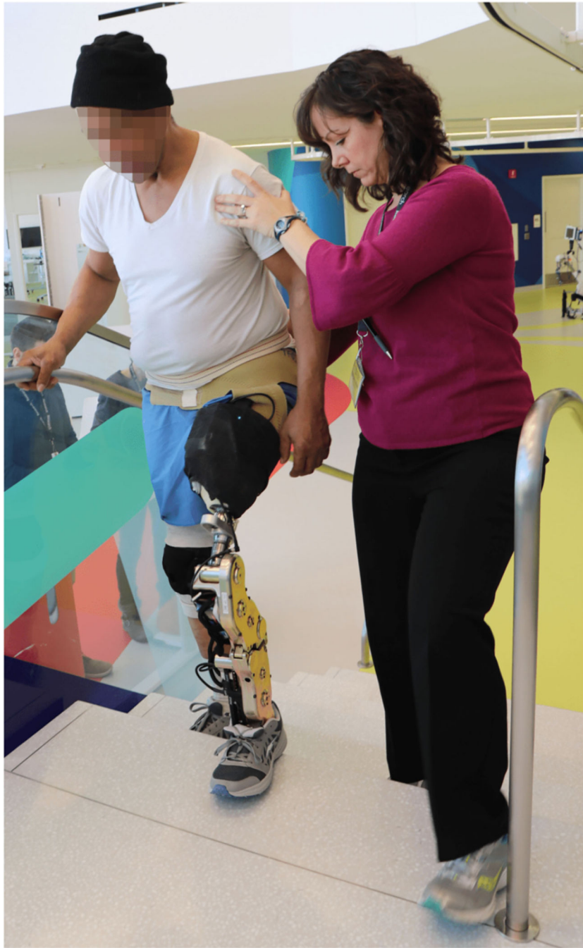
Fig. 1. Participant using the second-generation powered knee/ankle prosthesis from Vanderbilt University.
