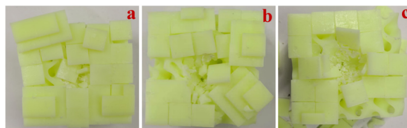
Figure 5. Experimental results. (a) B-C-A composite structure. (b) B-C-B composite structure. (c) B-C-C composite structure.
