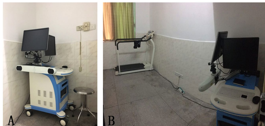
Figure 3. The gait system and the working place. (A) The gait analysis machine has about an area of 0.8 m × 0.8 m × 1.5 m. (B) The working place is located in the hospital near the doctors' office for the doctors to test patients.
