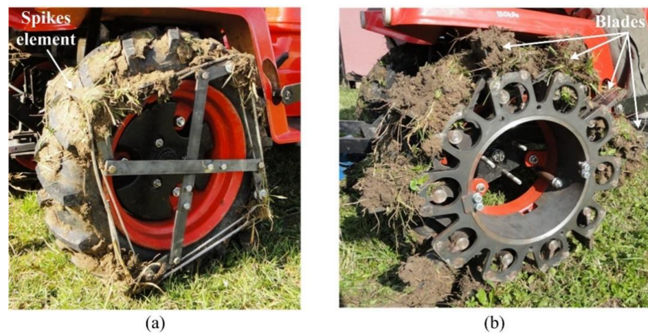
Figure 5. Special driving wheels covered with the soil under operation conditions on the grass plot: (a) spike tires; (b) blade wheels.
