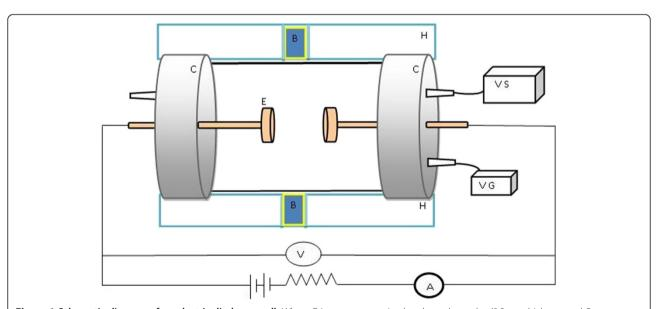
**Figure 1 Schematic diagram of an electric discharge cell.** Where E is two copper circular plane electrodes (0.2 cm thickness and 5 cm diameter), C is the reaction chamber (cylindrical Pyrex glass of 7 cm diameter and 15 cm length with 2 cm gap spacing, VS is the vacuum system, VG is the vacuum gauge, H is the sample holder, and B is cuvette place holder.
