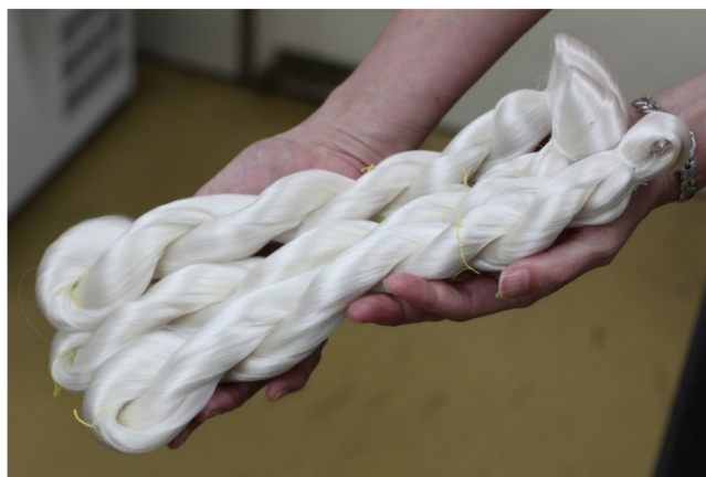
Figure 2. Picture of three bundles of the azido-functionalized raw silk fiber. Around 160 g of raw silk fiber was produced in total by rearing circa 1000 larvae of the F 1 hybrid, H06 × (Nichi509 × Nichi510). The larvae were fed AzPhe-containing diet (0.05 wt% in dry diet) on their third day of fifth instar until the start of spinning.
