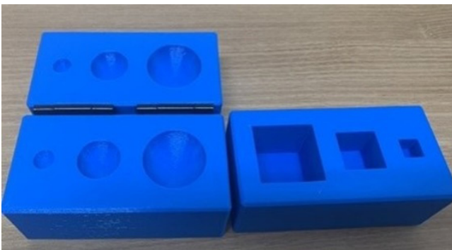
Fig. 2. 3D-printed molds to manufacture the phantom inclusion. The spherical mold consists of two halves with several cavities of different diameters (1, 2, and 3 cm), and the cubic mold consists of several cavities of different lengths (1, 2, and 3 cm).
