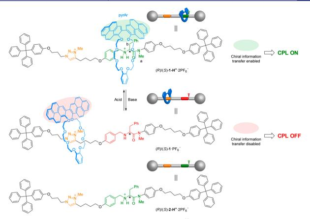
**Figure 2.** "On"–"off" switching of the CPL emission of rotaxanes (R)/(S)-1-H<sup>+</sup>·2PF<sub>6</sub><sup>-25</sup> based on the activation/deactivation of chiral information transfer from the thread to the luminescent macrocycle controlled by the acid/base-promoted shuttling of the macrocycle position on the thread.
