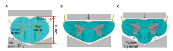
Figure 2. Finite Element Method analysis. (A) Before compression. (B) Anterior compression model and (C) anterior plus posterior compression model.
