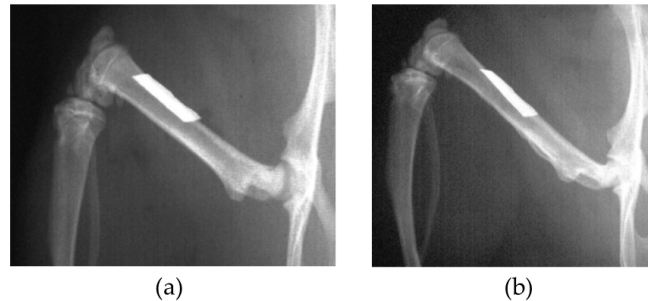
Figure 9. (a) Radiograph of left femoral bone just after BMG ribbon implantation; (b) Radiograph of femoral bone and BMG ribbon at 6 weeks after implantation. The size and shape of the ribbon have not changed from the original ones.
